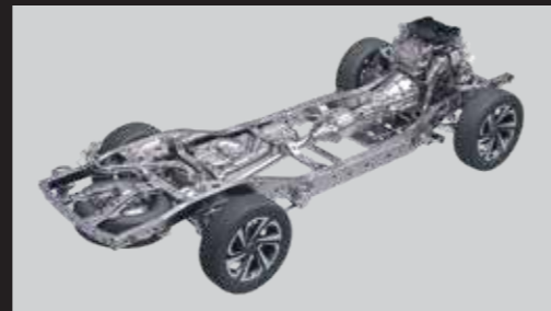
Larger Chassis Side Rails with increased inner side rail reinforcement allows 23% increase in torsional rigidity.
